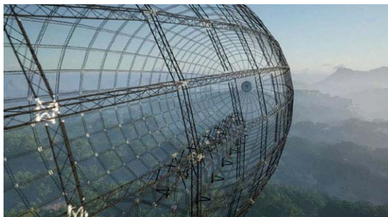
Figure 77: rigid structure of the airship
