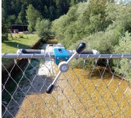
fig.: Tractel Dynarope, rope force measuring device
