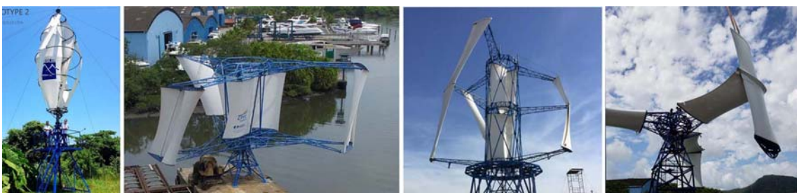
Figs.69, 70, 71, 72: Vertical-axis wind turbine prototypes from the research and development project carried out by CPFL, V/LEAF and Fiedler.
