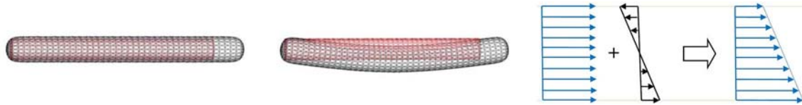
Fig.96: natural and initial states. Fig.97: deflected beam. Fig.98: Longitudinal stresses of the deflected beam.
