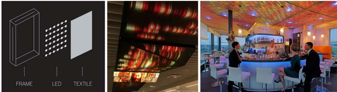
Fig. 128: Basic system: frame+LED+textile. Fig.129: Dynamic ceiling over fast lane. Brussels Airport. Fig.130: Bar ceiling installation. Brussels Airport.
