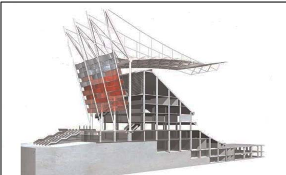
The Warsaw Stadium is notable (left) for being built above a volcano shape, its compression ring and the cables penetrating the membrane (right).
