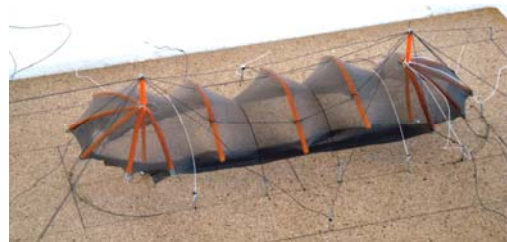
D. Veenendaal minimized the number of vertical supports under compression
