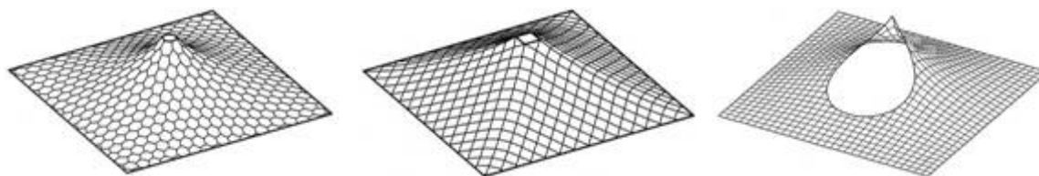
High point of a net with hexagonal (left), square mesh (middle) and square mesh with opening (right)
